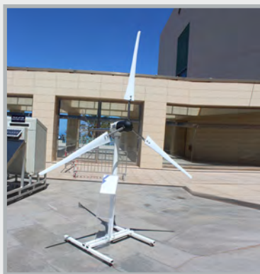
Small wind turbine blades in composite material « Resin and fiberglass » (1KW), CDER-2017
