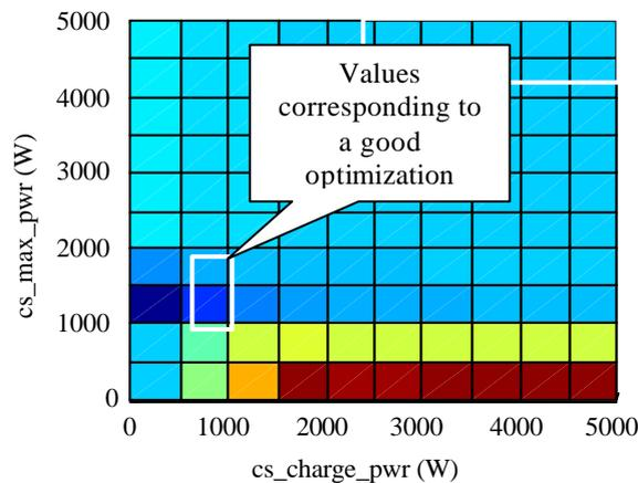
Fig. 8 : Computation of the parameters *cs\_max\_pwr* and *cs\_charge\_pwr* for the constant speed driving schedule
