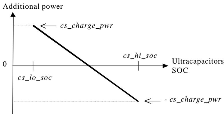
Fig. 6 : Computation of additional power for ultracapacitors SOC correction
