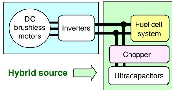
Fig. 2 : Structure of the vehicle drive train
