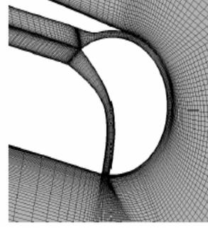
Fig. 3: Mesh around the trailing edge and inside the air jet ducts
