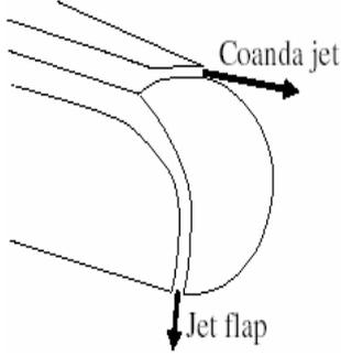
Fig. 1: WTEA airfoil trailing edge topology showing the air jet ducts
