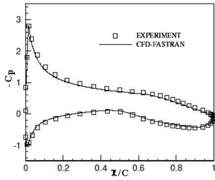
Fig. 4: Pressure coefficient profile for not-jet flow configuration obtained for  $Ma=0.25$ ,  $\alpha=5^\circ$  and  $Re_C=2 \times 10^6$
