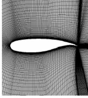
Fig. 2: Mesh around the WTEA airfoil
