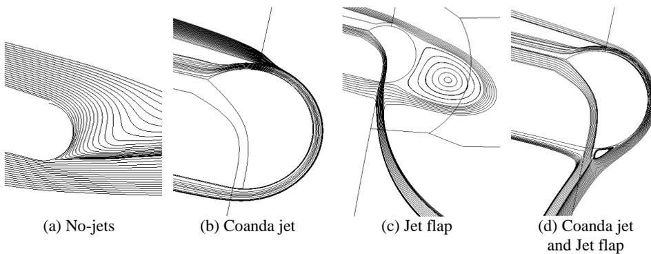
Fig. 7: Flow streamlines around the airfoil trailing and inside the jets ducts
