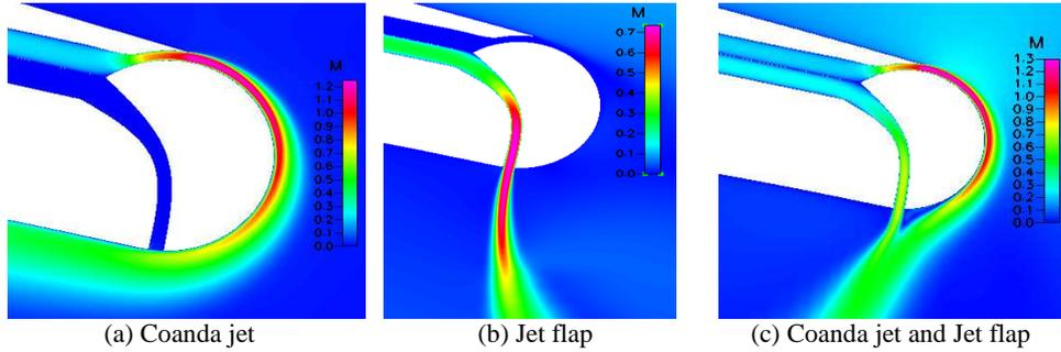
Fig. 6: Mach number distribution around the airfoil trailing edge for  $Ma=0.14$ ,  $\alpha=5^\circ$  and  $Re_C=10^6$
