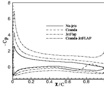
Fig. 5: Pressure coefficient profiles for different flow configurations obtained for  $Ma=0.14$ ,  $\alpha=5^\circ$  and  $Re_C=10^6$
