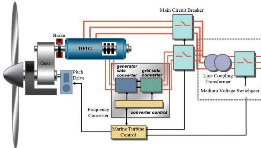
Fig. 6: Schematic diagram of a DFIG-based generation system
