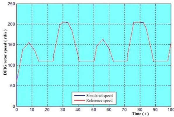
Fig. 9: The DFIG rotor speed and its reference
