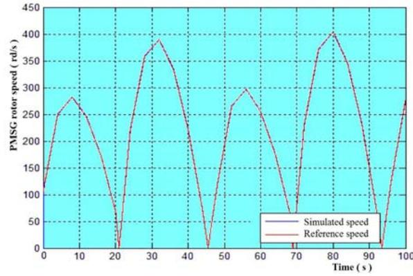
Fig. 11: The PMSG rotor speed and its reference
