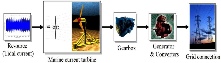
Fig. 2: Marine current turbine global scheme
