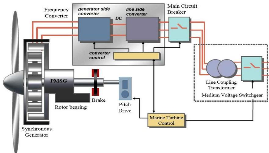
Fig. 7: Schematic diagram of a PMSG-based generation system
