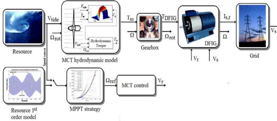
Fig. 8: Variable speed control for a DFIG-based MCT
