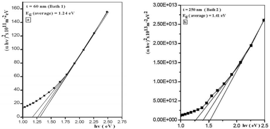
Fig. 5: Plot of  $(\alpha h\nu)^2$  vs  $(h\nu)$  of CIAS thin films prepared from chemical baths 1 and 2
