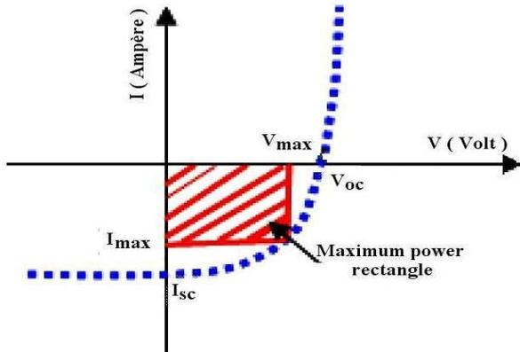
Fig. 3:  $I(V)$  characteristic of a solar cell
