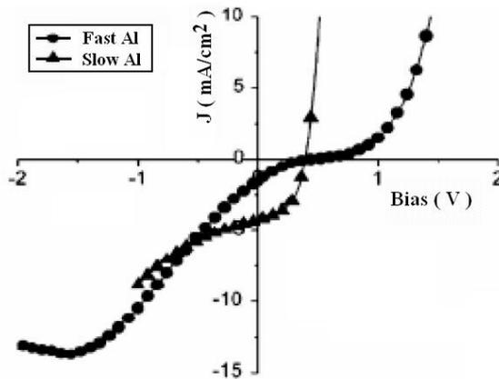
Fig. 5: Illuminated  $J(V)$  characteristics of a P3HT-PCBM solar cell with Al deposited at an extremely fast evaporation rate (200 nm/5 s) and at a slow evaporation rate (200 nm/100 s) [6]
