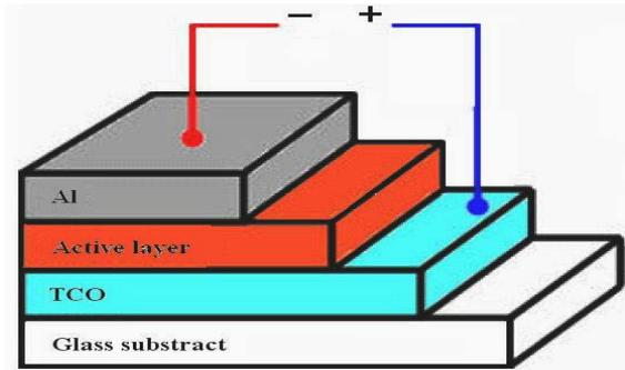
Fig. 2: Structure of the hybrid solar cell
