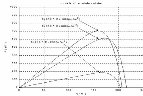
Fig.4. Effect of solar radiation and temperature on PV generator power
