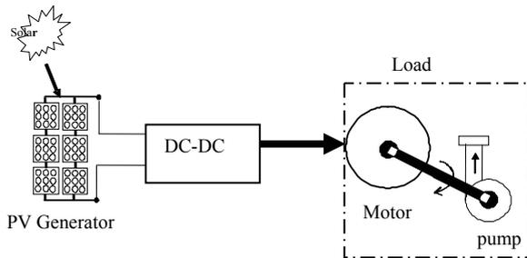
Fig.1: Schematics of a photovoltaic pumping system
