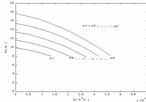
Fig.2: H-Q Characteristics centrifugal pumps with various speeds w
