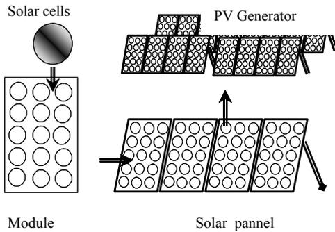
Fig. 3. Photovoltaic generator hierarchy
