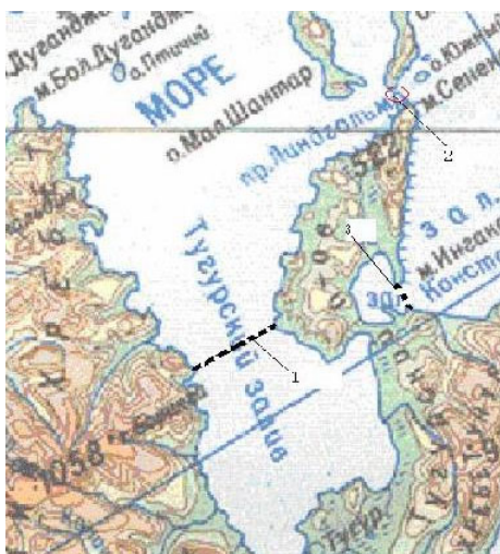
Fig. 8. The tidal power station in the narrowness of Tugursky Bay. The width of the strait is 15 km. The maximum rise of tide is 10.1 m, the average rise of tide is 8.6 m. The area of the exploitable part of the bay is 1400 km 2 . The maximum possible power of TPS is 19.4 GW. The maximum average annual production is 48 billion kwhr/yr. 1 – the site of the units of the proposed TPP, 2 – zone of arrangement of the first pilot unit of large capacity. 3 – possible TPP to produce basis power.
