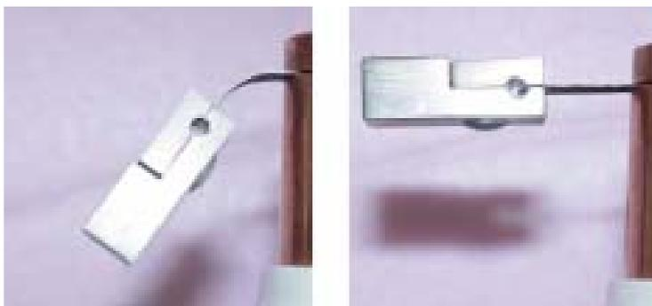
Figure 2. Shape memory actuator alloys under development at the University of Central Florida.
