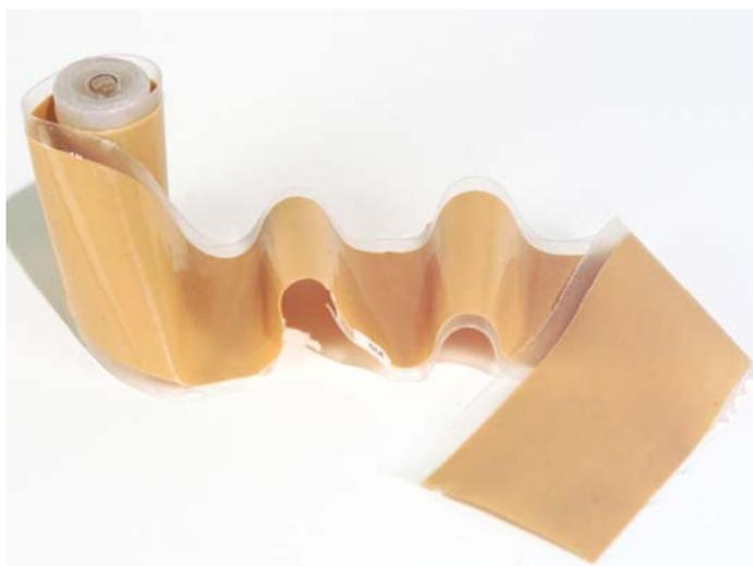
Figure 3. FSEC developed chemochromic hydrogen sensing and detection materials.
