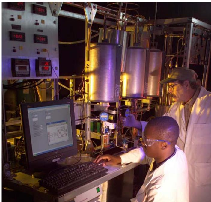
Figure 1. Pilot plant at FSEC for the production of hydrogen by catalytic reformation of hydrocarbon fuels and renewable feedstock.
