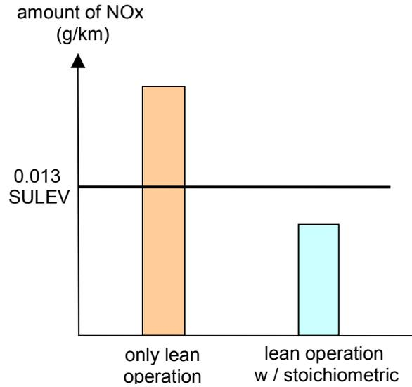
Fig.8 Effect of lean operation with stoichiometric operation
