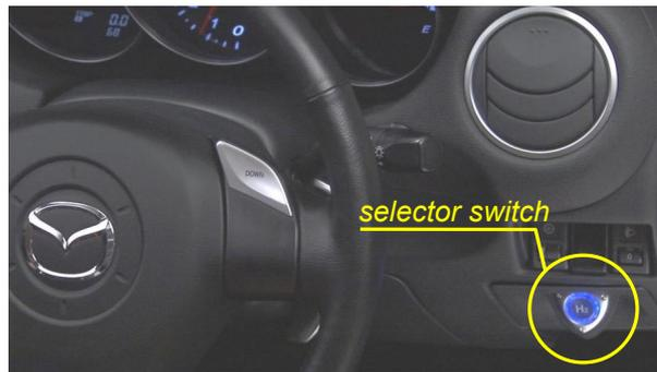
Fig.10 Selector switch for hydrogen/gasoline
