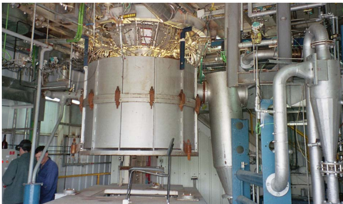
Figure 5: SOLZINC pilot plant in operation: The product gas of pilot solar reactor in the middle is quenched with recycled cold product gas in the vertical chamber on the right, before it passes a cyclone for separation of the Zn-dust.
