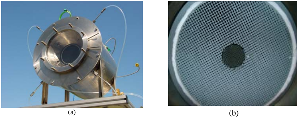
Figure 3: (a) Front view of the first solar water-splitting receiver-reactor, (b) Small-scale honeycomb coated with redox material (black) in the centre of the reactor ready for testing.
