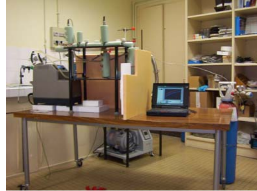
Figure 2 : photograph of the experimental setup used to measure PIS impedances.
