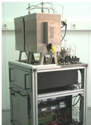
Figure 4: Test unit for gas phase desulphurisation experiments
