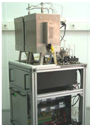
Figure 4: Test unit for gas phase desulphurisation experiments
