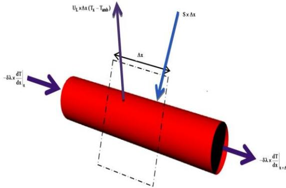
Fig. 3: Energy balance on fin element
