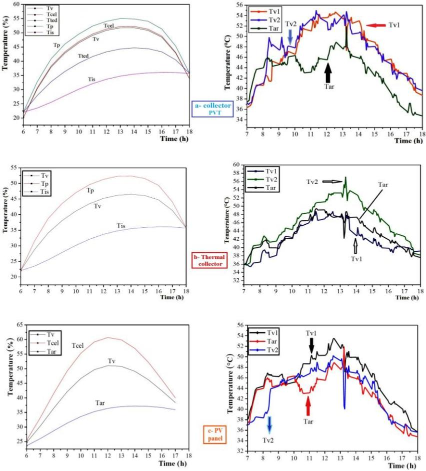
Fig. 5: Distribution of temperature in different collector
