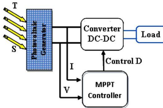
Fig. 3: Photovoltaic systems
