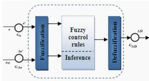
Fig. 5: Basic structure of fuzzy logic control
