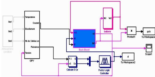
Fig. 6: Model SIMULINK of MPPT controller flou
