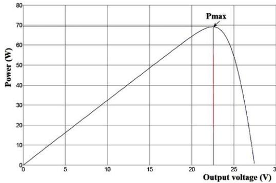
Fig. 2: Power curve under constant irradiation and temperature
