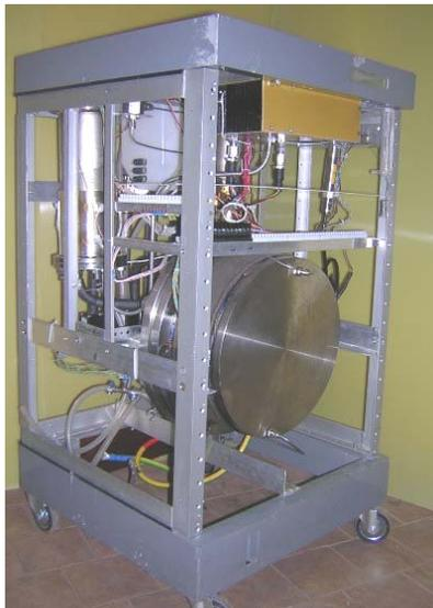
**Fig. 12.** 1.5 m<sup>3</sup>/hour hydrogen generator operated up to 30 bars (KI).
