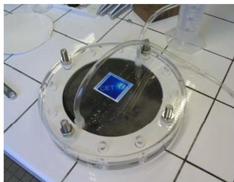
Figure 7 : photograph of a  $250\text{ cm}^2$  MEA Nafion®117/Pt kept in water after Pt deposition.
