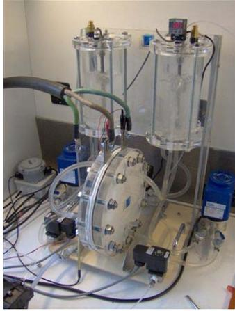
**Figure 8** : typical monosell of nominal scale used to test MEAs performances (CETH).
